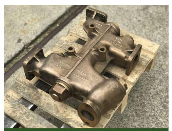
Using a series of converging and diverging cones, an injector is used to deliver cold water into the boiler against its own pressure, using its boiler steam with no moving parts.
