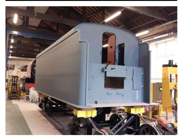
The third of the big items for delivery this year is the tender frames. Continued progress has been made on the tender frames at I D Howitt of Crofton, Wakefield, with the axleboxes machining completed and further work on brake and hand brake components. The tender tank is already at in Darlington and is poised to be attached to the frame after its arrival. The wheels, also at DLW in readiness, will require balancing.
